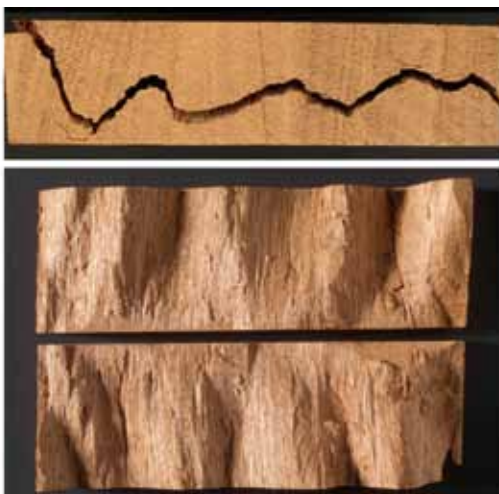
Figure 2. Sinuous course of the radial longitudinal split and the resulting pattern of peaks and valleys on the radial surface of the two separated pieces, for example in African Bilinga wood ( Nauclea diderrichii )
