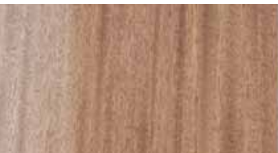
Figure 1a. Alternating light and dark strips caused by different reflection of incident light, for example in Sapele ( Entandrophragma cylindricum )
