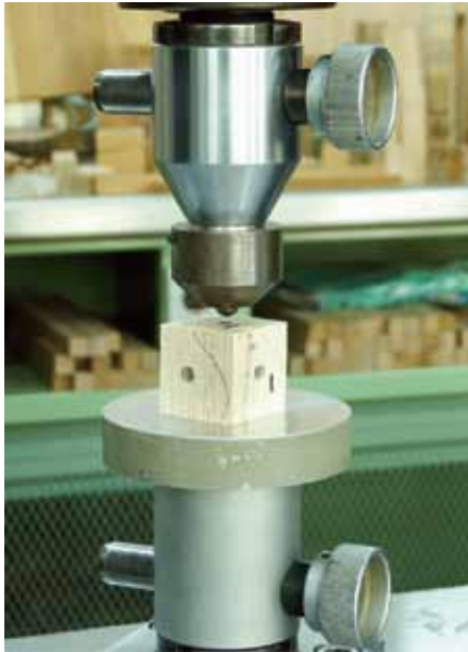
Figure 9. BRINELL hardness test
